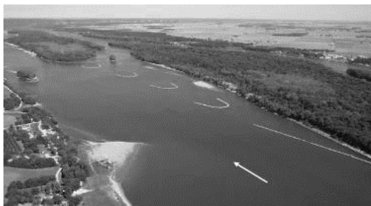
Figura 2.12-3 Exemplu de camp chevroane (sursa: Inland Navigation Channel Training Works ASCE MOP)
