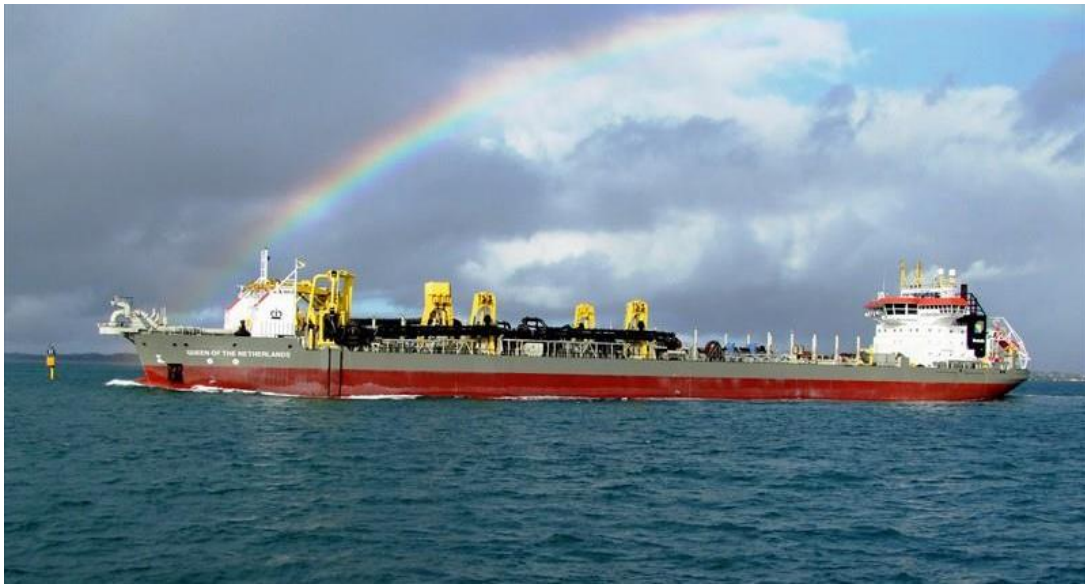
Fig. 2.8 – Nava a companiei Boskalis – Queen of the Netherlands – cu o capacitate de 35.500 mc (marine traffic.com)
